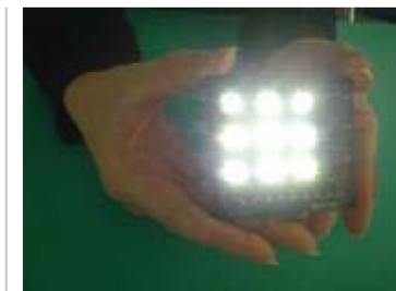
Demonstration using nine pieces of the latest white LEDs: a luminous flux of 90 lm was achieved at an
