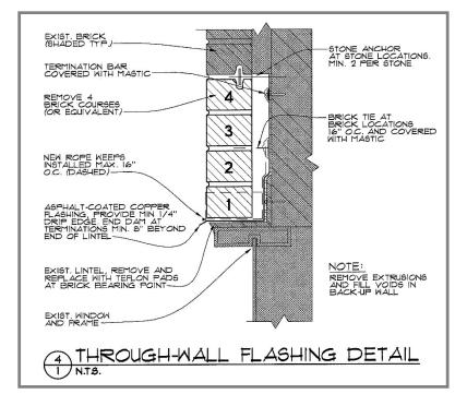
Also: re-anchor stone, rebuild inner wythe, and replace wood joist ends
